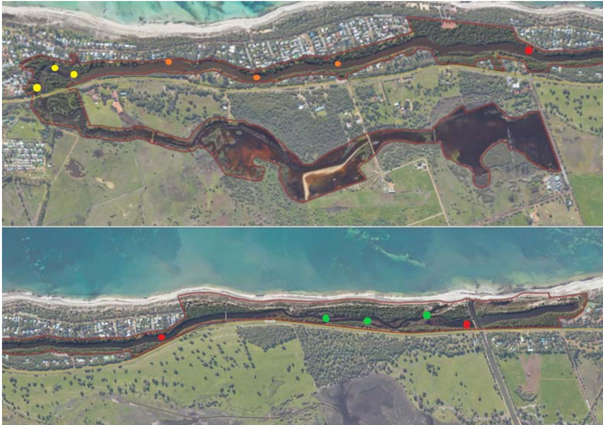
Figure 8. Acid sulphate soil and monosulfidic black ooze (MBO) presence in Toby Inlet sediments. Yellow markers show sand-dominated sediments with potential acid sulphate soils but no MBOs found in 2007 study. Orange sites show MBOs and potential acid sulphate soils in 2007 study. Green sites show no potential acidity or MBOs found in 2009 study. Red sites show MBOs and potential acid sulphate soils in 2009 study.
